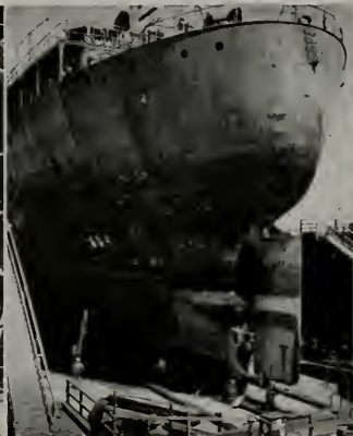
Center below: View of the Mobilube on drydock at Bethlehem's San Francisco Yard. Upper half of temporary planking of "soft patch" has been removed revealing temporary frame. Lower right: Mobilube's huge reduction gear being inspected in Bethlehem's machine shop.
